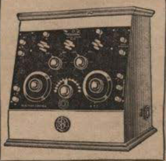
The "DUNHAM" 3-Valve Receiver.
